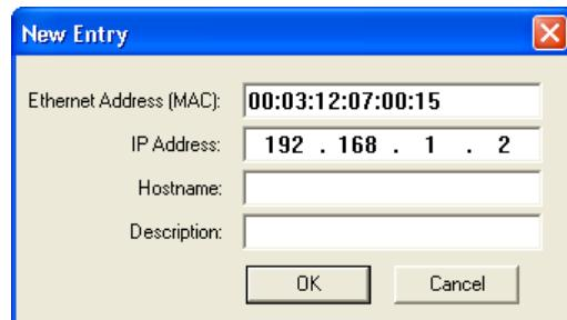
The new entry is indicated in the Relation List. The predefined IP parameters are assigned to the measuring system with the next DHCP request. The result of this assignment is registered into the Request History:
