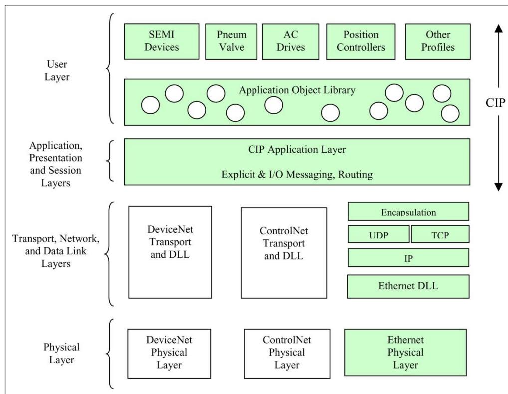
Figure 1: Relations between CIP™, DeviceNet™, ControlNet™ and EtherNet/IP™
