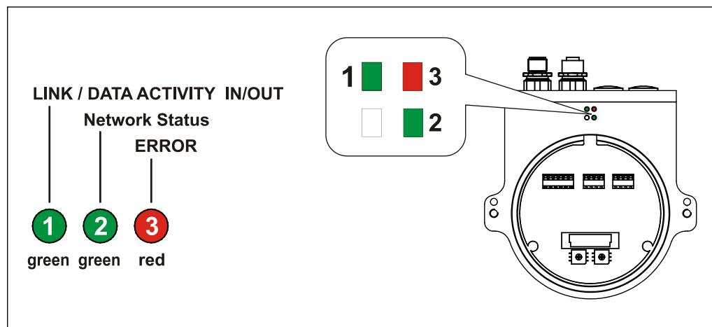
Figure 4: EtherNet/IP™ diagnostic LEDs
