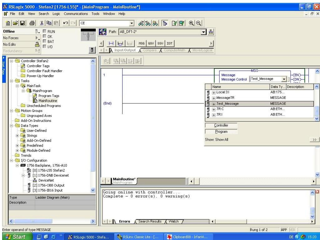
5. Configure the message in the Message Configuration dialog box --> Configuration tab as follows. Following example reads the position value, attribute 0x03 Position Value, from the Position Sensor Object 0x23:
