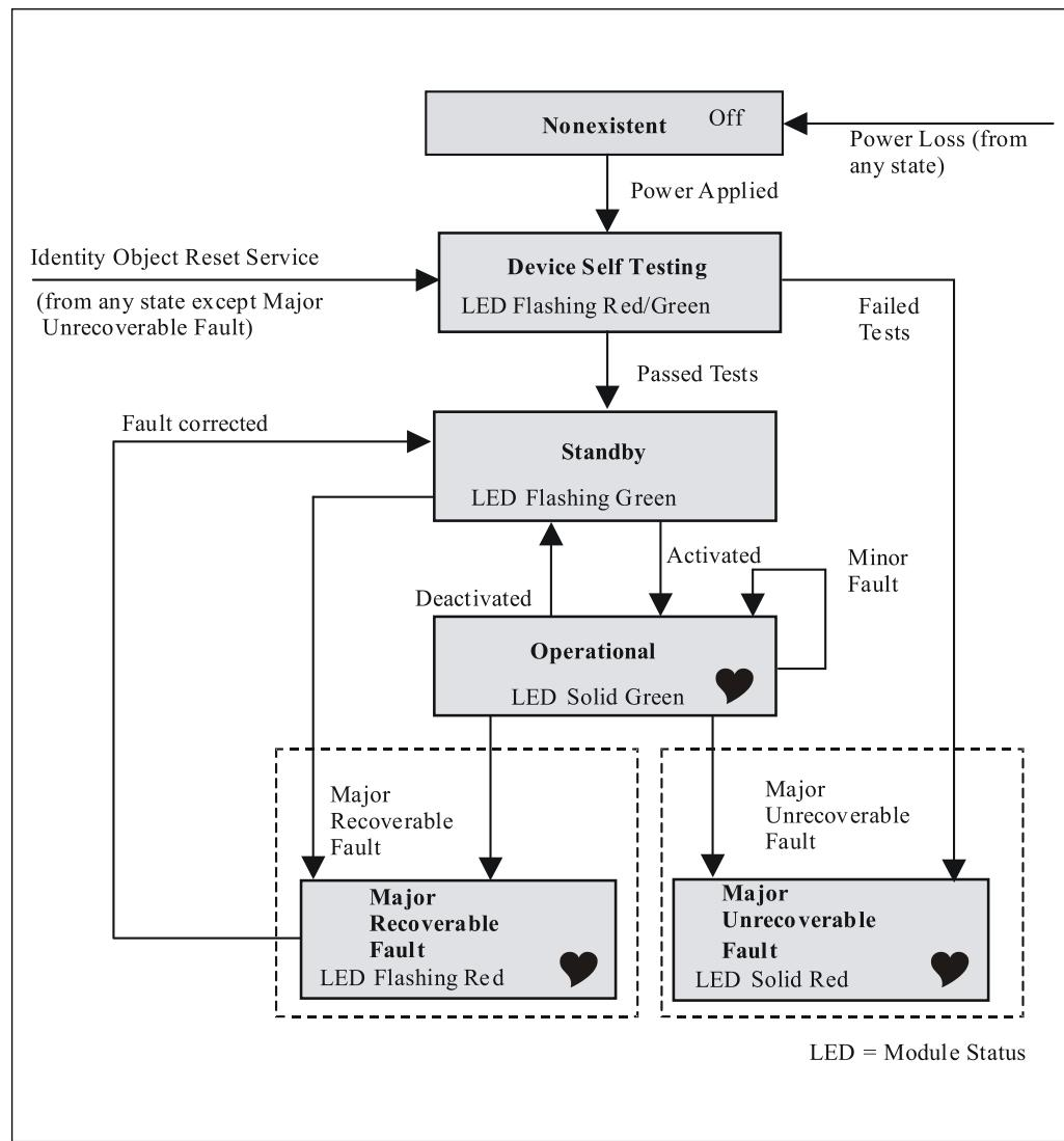
Figure 6: State Transition Diagram [Source: ODVA™ EtherNet/IP™ Specification]
