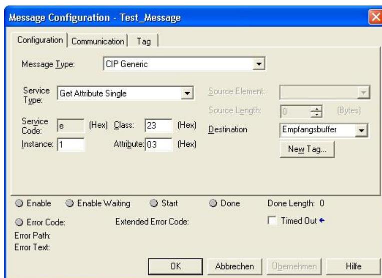
6. Bind the configured message with the created module in the Message Configuration dialog box --> Communication tab:
