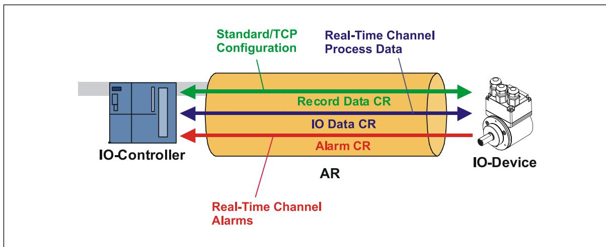
**Figure 3: Device communication**
