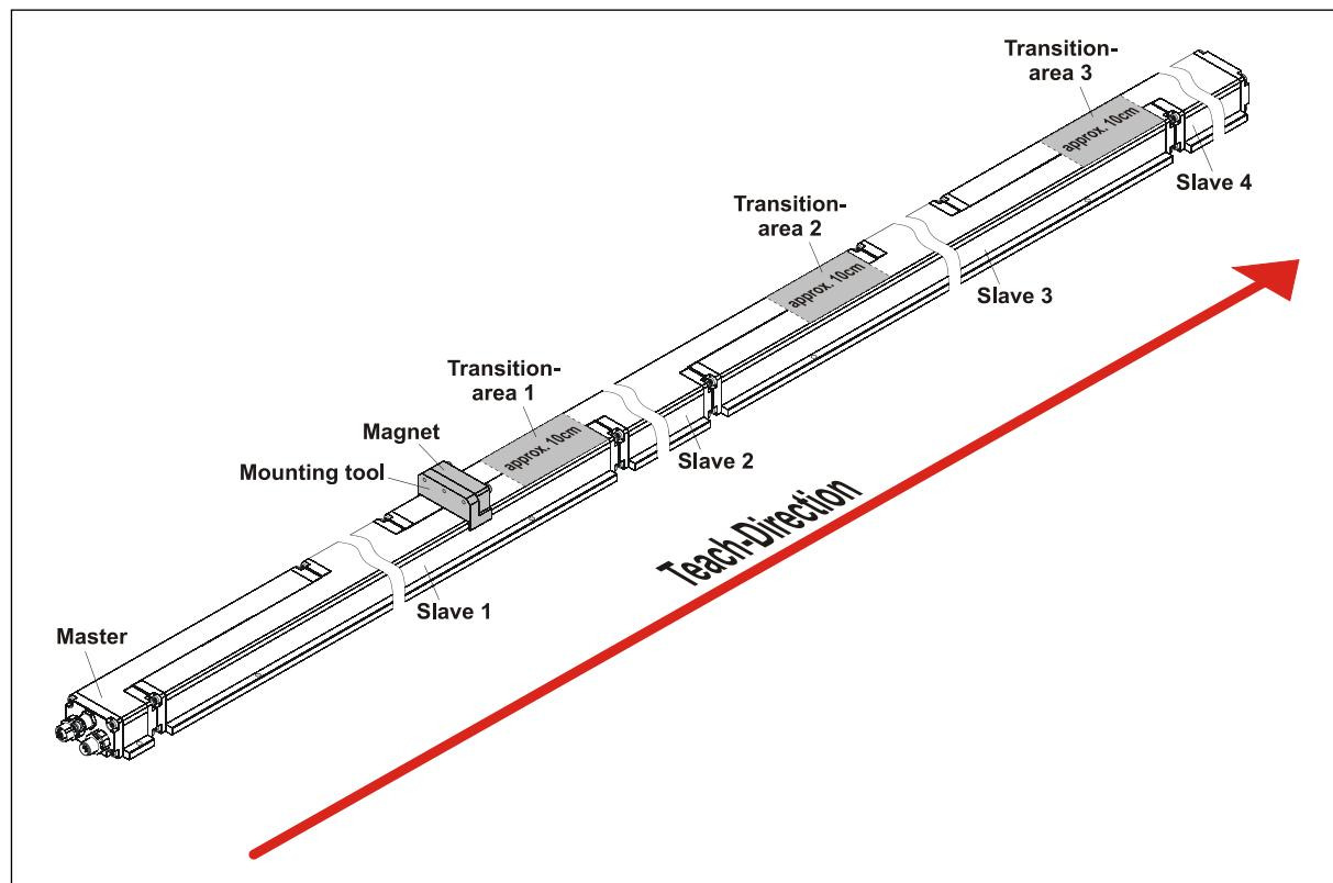
Figure 5: Configuration example with four slaves
