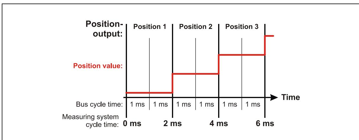
Figure 5: Example for position value output without interpolation
