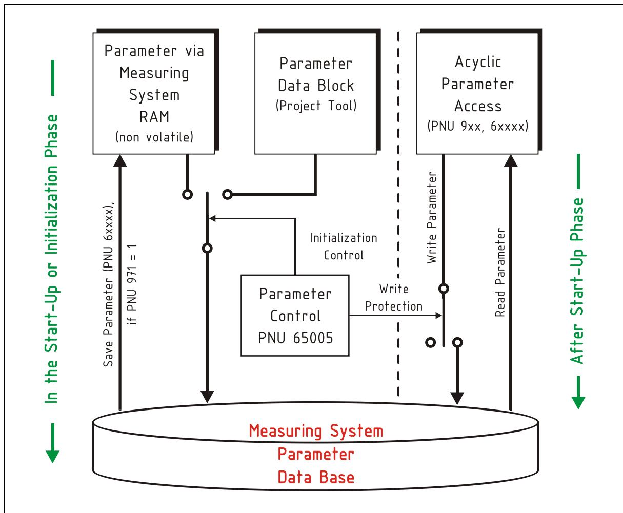
Figure 4: Parameter access and initialization (simplified functional representation)
