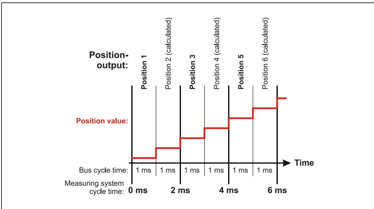
Figure 6: Example for position value output with interpolation
