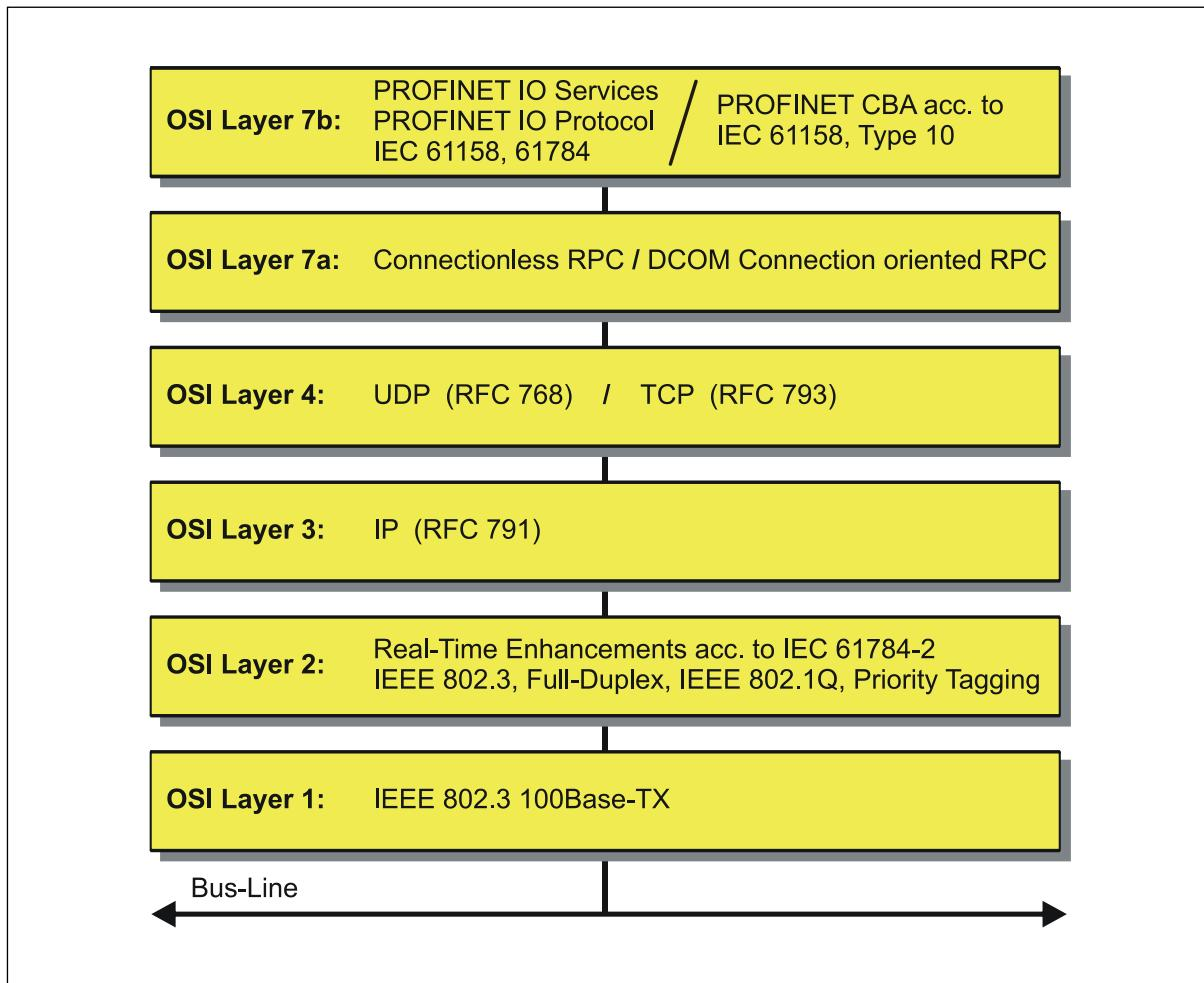
Figure 1: PROFINET organized in the ISO/OSI layer model
