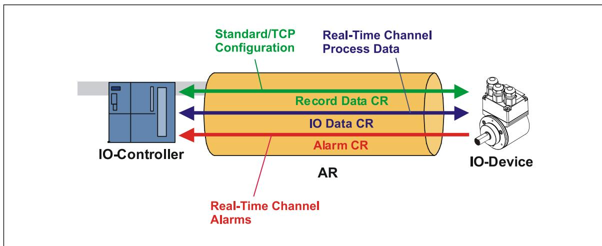
Figure 3: Device communication
