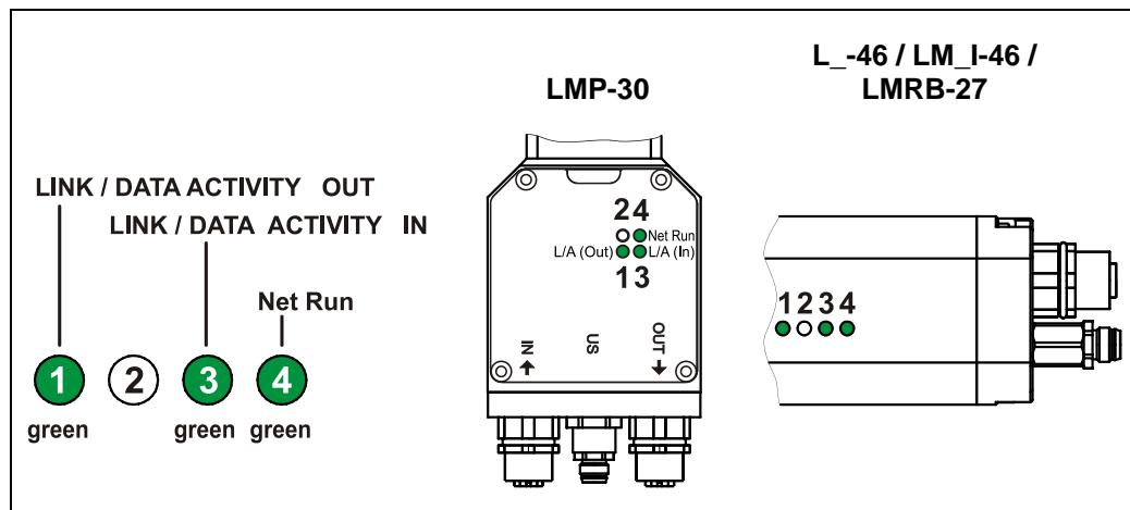
Abbildung 9: EtherCAT Diagnose-LEDs
