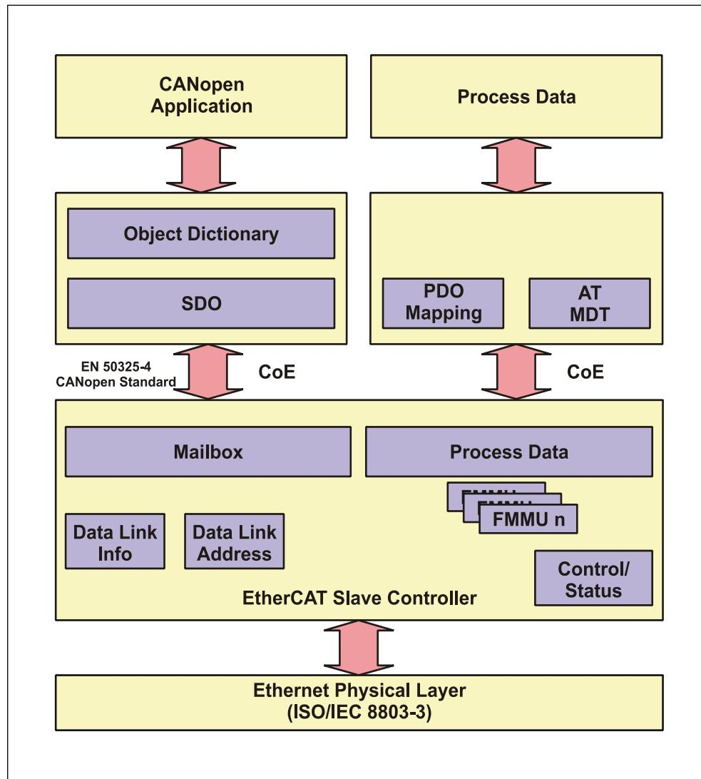
Figure 3: CANopen over EtherCAT communication mechanism
