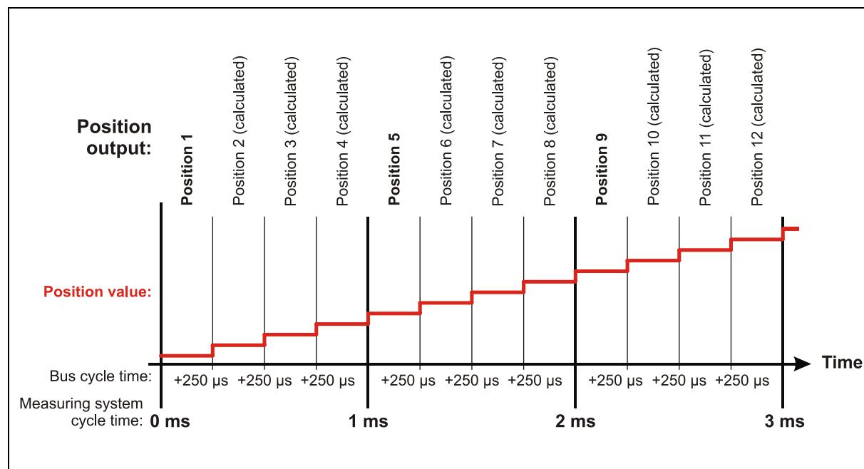
Figure 11: Example for position value output with interpolation
