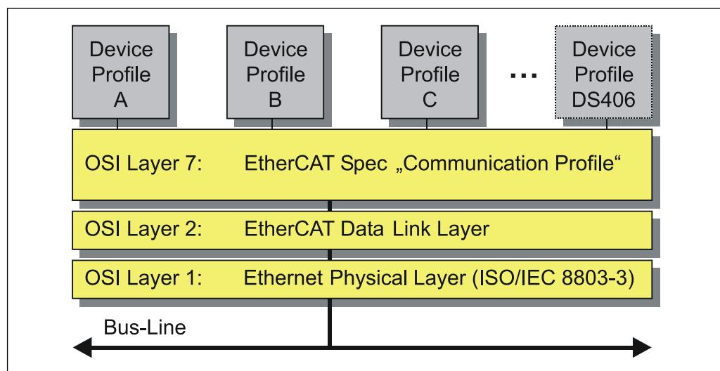
Figure 5: EtherCAT organized in the ISO/OSI layer model
