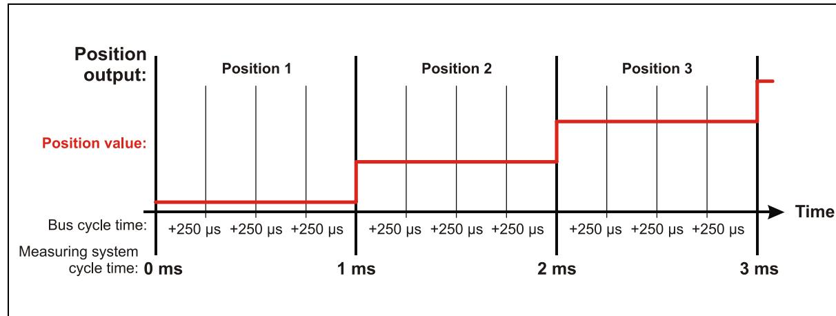
Figure 10: Example for position value output without interpolation
