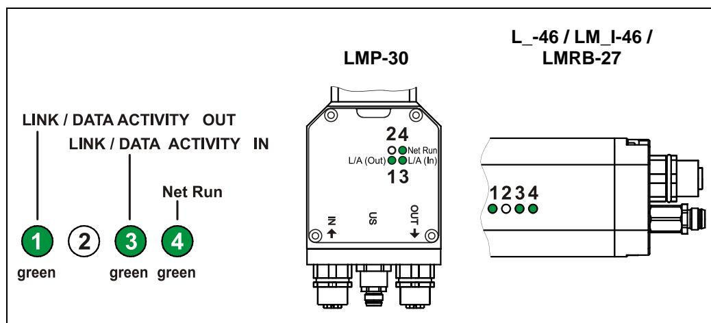
Figure 9: EtherCAT diagnostic LEDs
