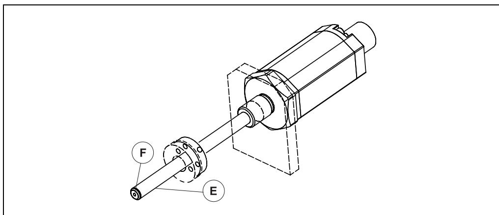
**E:** Horizontal inserted rods > 1.5 m long should be supported and a position sensor open to the extent be used.
