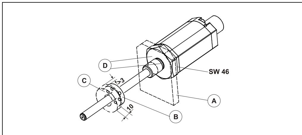
**A:** The linear transducer is fixed directly with the thread or a nut/mother with the mounting plate, with one attraction moment of < 50 Nm.
