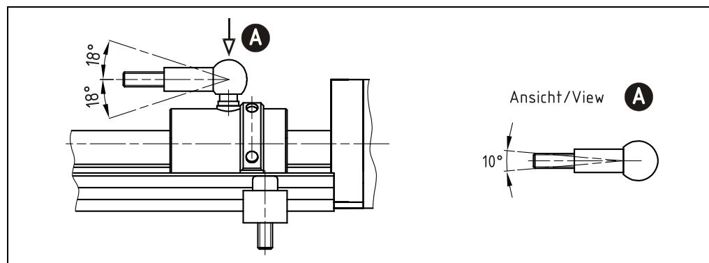
The exact of the measured value depends also on the symmetry of magnetic field geometry. If no captive-sliding magnet is used, the position sensor must be led exactly in axial direction to the measuring body. The admissible maximum distance between position sensor and measuring body may not be exceeded:
