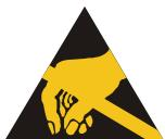
means that appropriate ESD-protective measures are to be considered according to DIN EN 61340-5-1 supplementary sheet 1.
