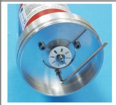
Fasten mounting flange, on the side of the O-ring, with the encoder. For this purpose the three cheese-head screws M4x8 should be used.
