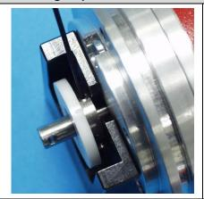
Attach mounting gage to the encoder:
