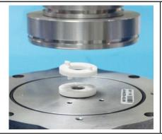
Insert clutch disc onto the housing of the cable traction box. Place encoder with flange ring and clutch disc onto the O-ring of the cable traction box housing.
