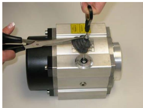
2. Cut open the bellows and remove it
