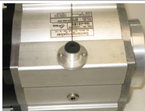
6. Press tightly the rubber ring onto the flange
