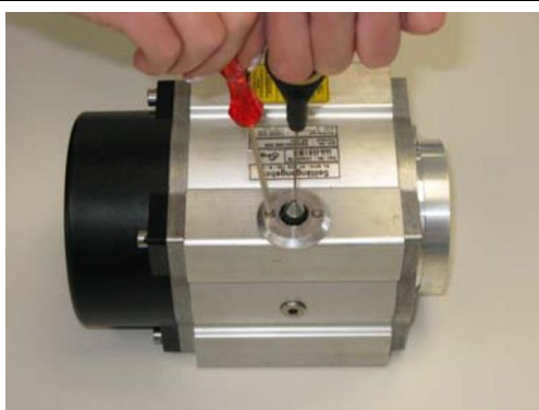
3. Remove flange for version with bellows
