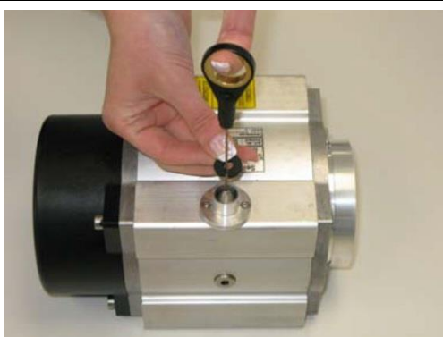
5. Fix nozzle with rubber ring inside the flange
