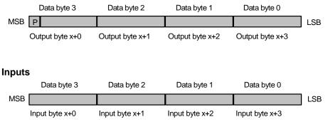
The preset adjustment value transferred in data bytes 0 - 3 is accepted as the position value with the leading edge of bit 32 (=bit 7 of data byte 3).
