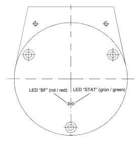
The encoder is equipped with two LEDs. One red LED (BF) for indicating errors and one green LED (STAT) for indicating status information.
