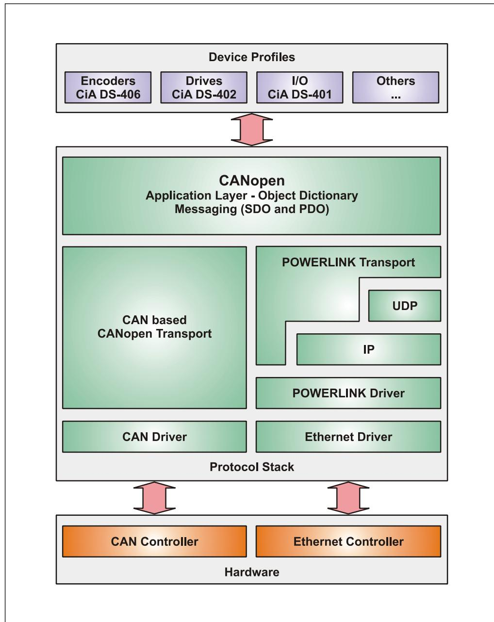
Figure 4: Virtual EPL / CANopen software architecture
