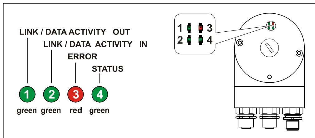
Figure 15: POWERLINK diagnostic LEDs
