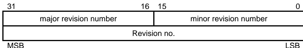
The major revision number identifies a specific device behavior. If the device functionality is expanded, the major revision is incremented. The minor revision number identifies different versions with the same device behavior.
