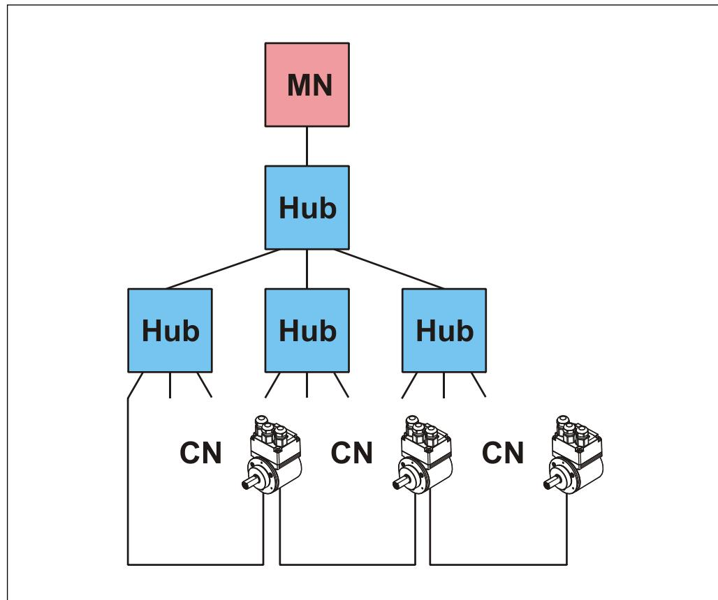
Figure 12: Star- and line-topology in one EPL network
