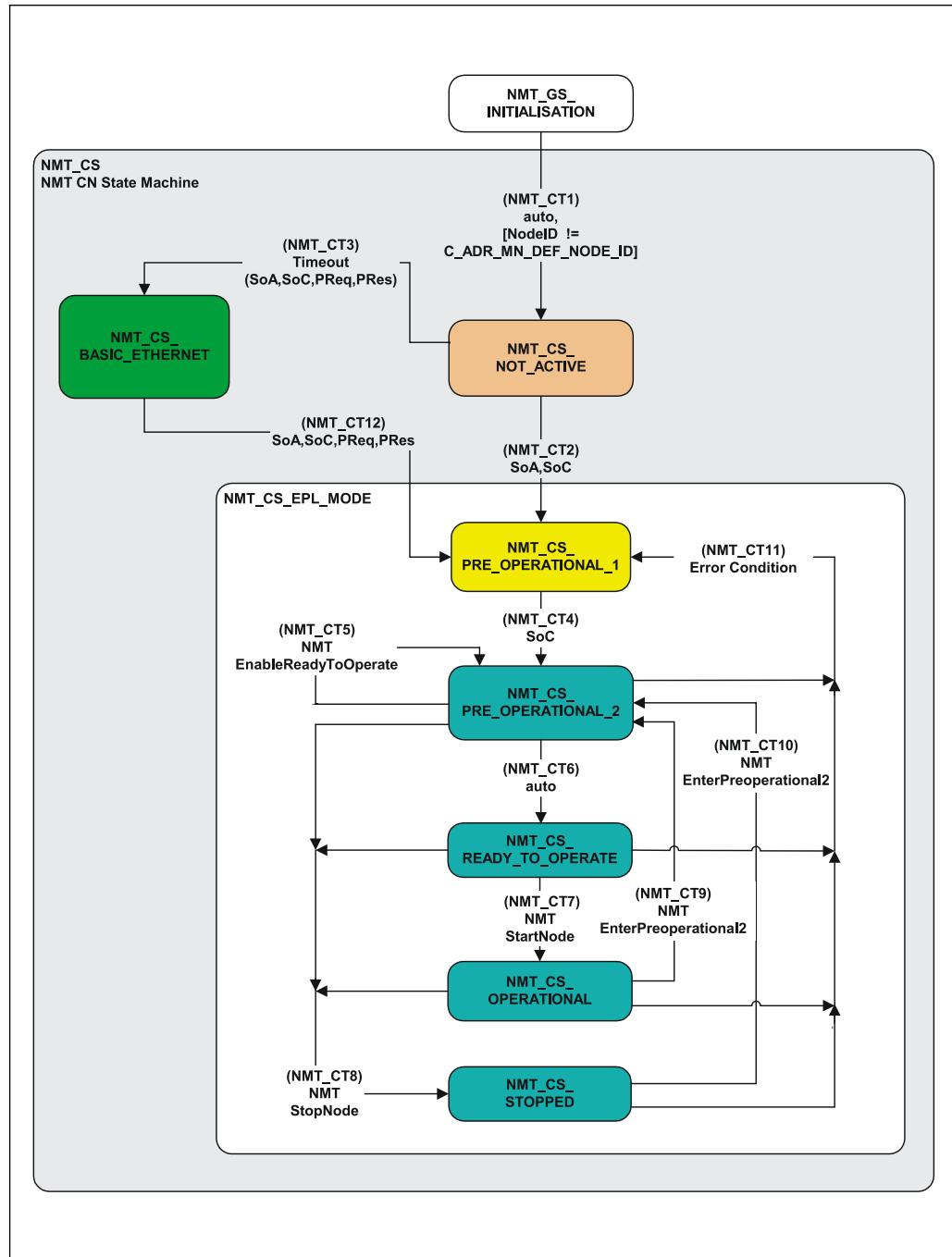
Figure 11: NMT CN State Machine [Reference: EPSG Powerlink Specification]
