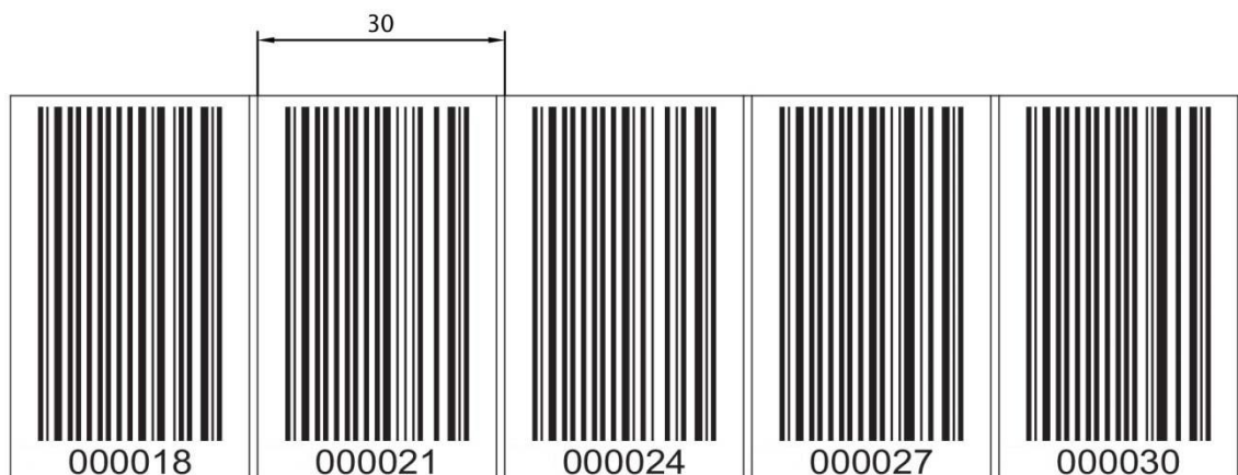
Figure 11.2: Checking the print results of the BCB G30 repair kit (30 mm grid)
