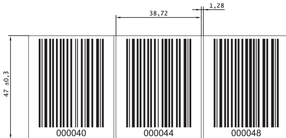
Figure 12.11: Dimension drawing barcode tape BCB G40 with 40 mm grid (all dimensions in mm)
