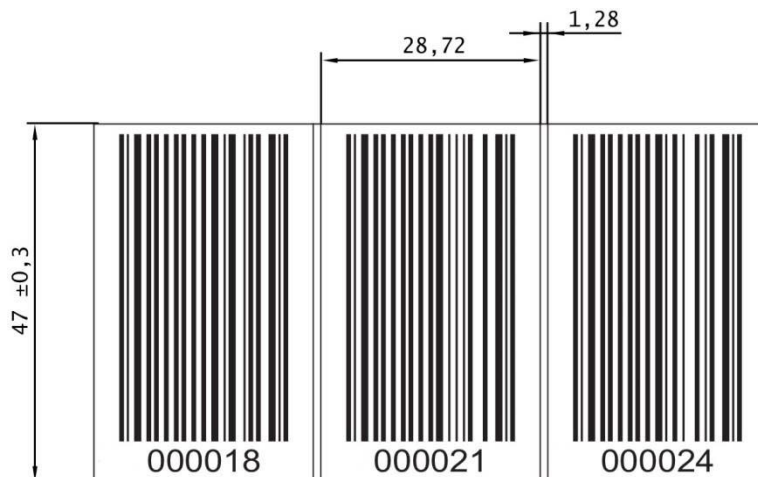
Figure 12.12: Dimension drawing barcode tape BCB G30 with 30 mm grid (all dimensions in mm)
