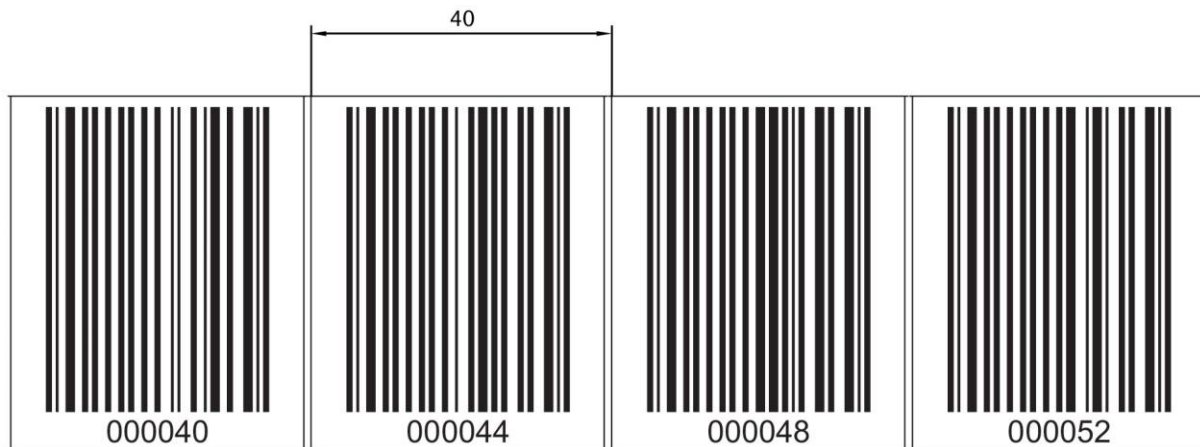
Figure 11.1: Checking the print results of the BCB G40 repair kit (40 mm grid)
