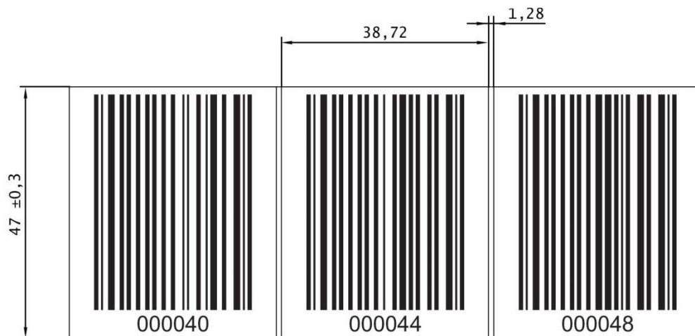
Figure 12.11: Dimension drawing barcode tape BCB G40 with 40 mm grid (all dimensions in mm)
