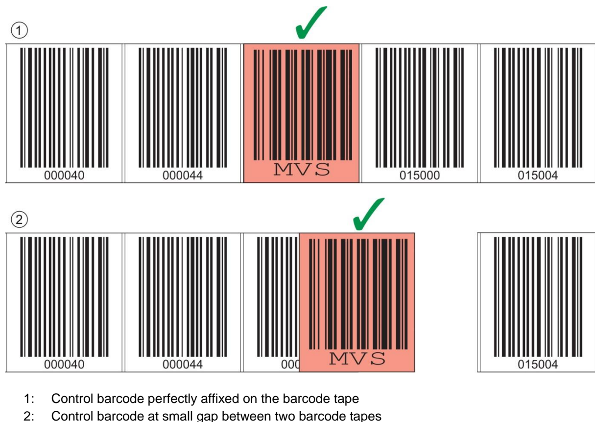
Figure 3.11: Correct positioning of the control barcode
